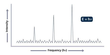
These discrete peaks occur as a repeatable frequency pattern corresponding to a specific substance. This general application is used for the identification of an unlimited number of atoms, molecules, and substances since they all have specific frequencies and patterns.
